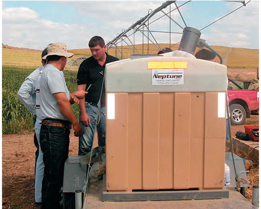
UNDER THE PIVOT. A chemigation system from Neptune Chemical Pump Company is shown mounted on a trailer for moving easily between multiple center pivot watering systems.
