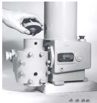
FIGURE VII VALVE CARTRIDGE REMOVAL, PVC HEAD PUMP
