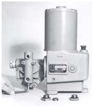
FIGURE VI VALVE CARTRIDGE REMOVAL, METAL HEAD PUMP
